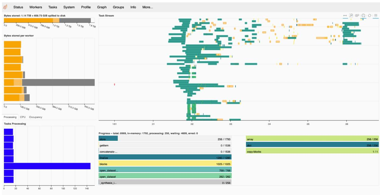
When the number of chunks is increased to 3840 the Dask dashboard below shows that no spilling to disk occurs.
